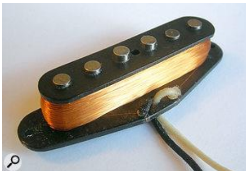
Figura 12 - Captador magnético (sound on sound: https://www.soundonsound.com/techniques/guitar-technology )
